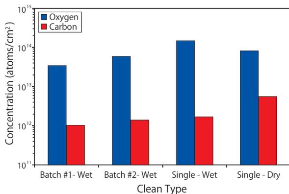
Fig. 3: Interface doses for Carbon and Oxygen atom after Wet & Dry cleans, no pre-bake, cold load, with 150nm Si deposition at 650°C ( 2hours queue time)
