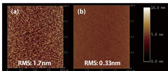
Fig. 6: AFM scans of (a) one-step SiCP film with TF-2 (not optimized process for gas phase particle) and (b) CDE SiCP film with TF-2 (optimized process)
