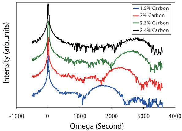
Fig. 7: XRD results of SiCP film with TF-2: up to 2.3% C substitutional profiles are obtained
