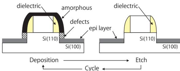
Fig. 5: Scheme of cyclical deposition and etch
