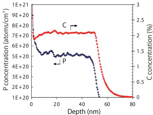
Fig. 8 SIMS profile of SiCP film with TF-2
