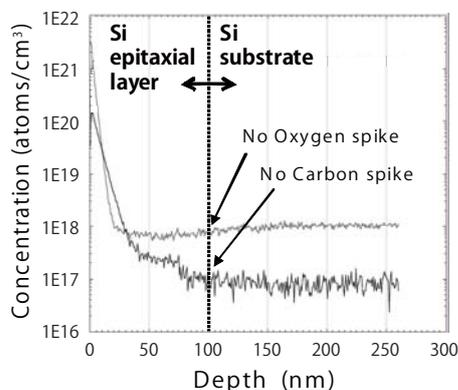
Fig. 4: SIMS depth profile with proper wet clean and minimized temperature (775°C) H<sub>2</sub> pre-bakes for epitaxy
