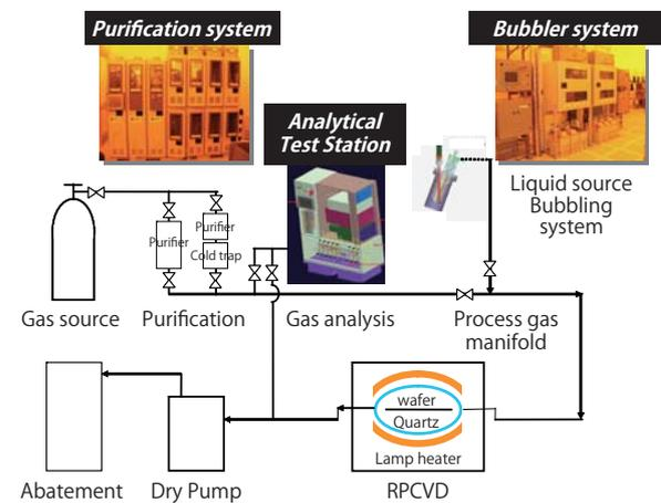
Fig. 2: The system of gas purification and gas delivery
