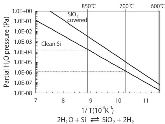
Fig. 1: Formation of SiO<sub>2</sub> as a function of H<sub>2</sub>O partial pressure and temperature: reconstructed from reference<sup>3)</sup>
