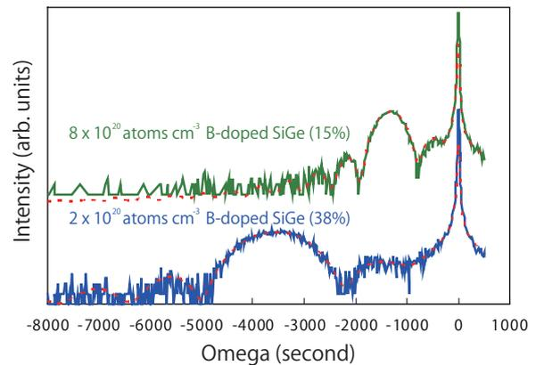
Fig. 9: XRD results of SiGeB film with TF-2: up to 38% Ge substitutional profiles are obtained
