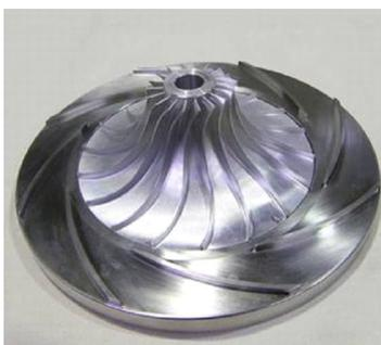
Fig. 2 Photograph of the first stage impeller and vaned diffuser
